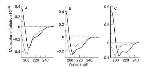
**Fig. 4.** Circular dichroism spectra of (A) TKYKQRNGWSHKDLLRSHLKP (169–190); (B) ELYKEKALSVETEKLLKYLEAV (211– 232); and (C) HLA-DR3 RPDAEYWNSQKDLLEQKRGR in H<sub>2</sub>O (---) and 50:50 TFE/H<sub>2</sub>O (—). Concentration 8.0–  $8.5 \times 10^{-4}$  M.
